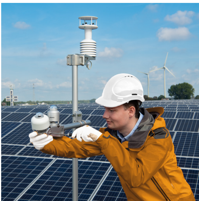
Figure 2 Typical use of pyranometers at PV power plants. The above picture shows two SR200-A1 pyranometers, one tilted for Plane of Array (POA) measurement, and another mounted horizontally for Global Horizontal Irradiance (GHI) measurement.
