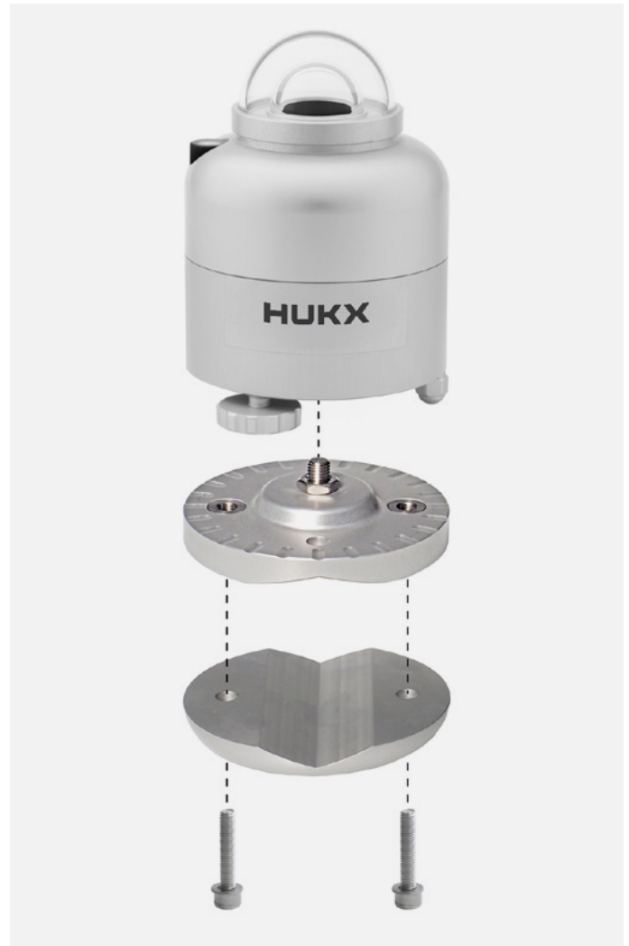
Figure 5 Optional LM01 spring-loaded leveling mount (only upper part) and TLM01 tube leveling mount (upper and lower parts) for SR200-A1 and SR100-A1. Spring-loaded leveling is a major time-saver during installation.
