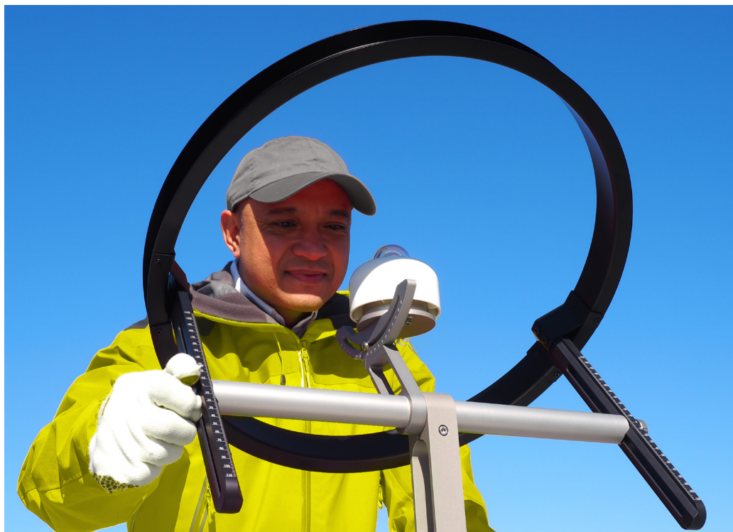
Figure 0.2 Installation of the SHR03 shadow ring with a Hukx pyranometer is easy.
