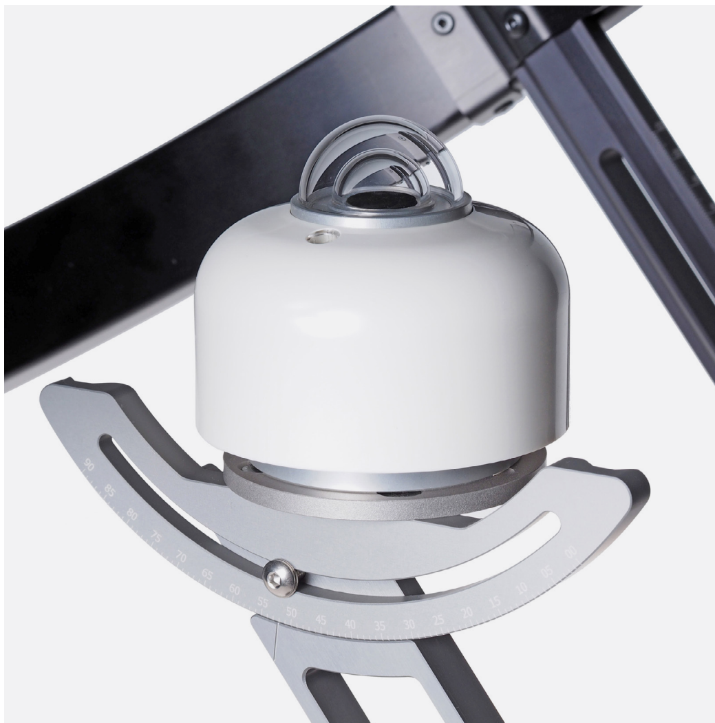
Figure 0.3 Pyranometer example: SR200-D1, combined with SHR03 forming a diffusometer.
