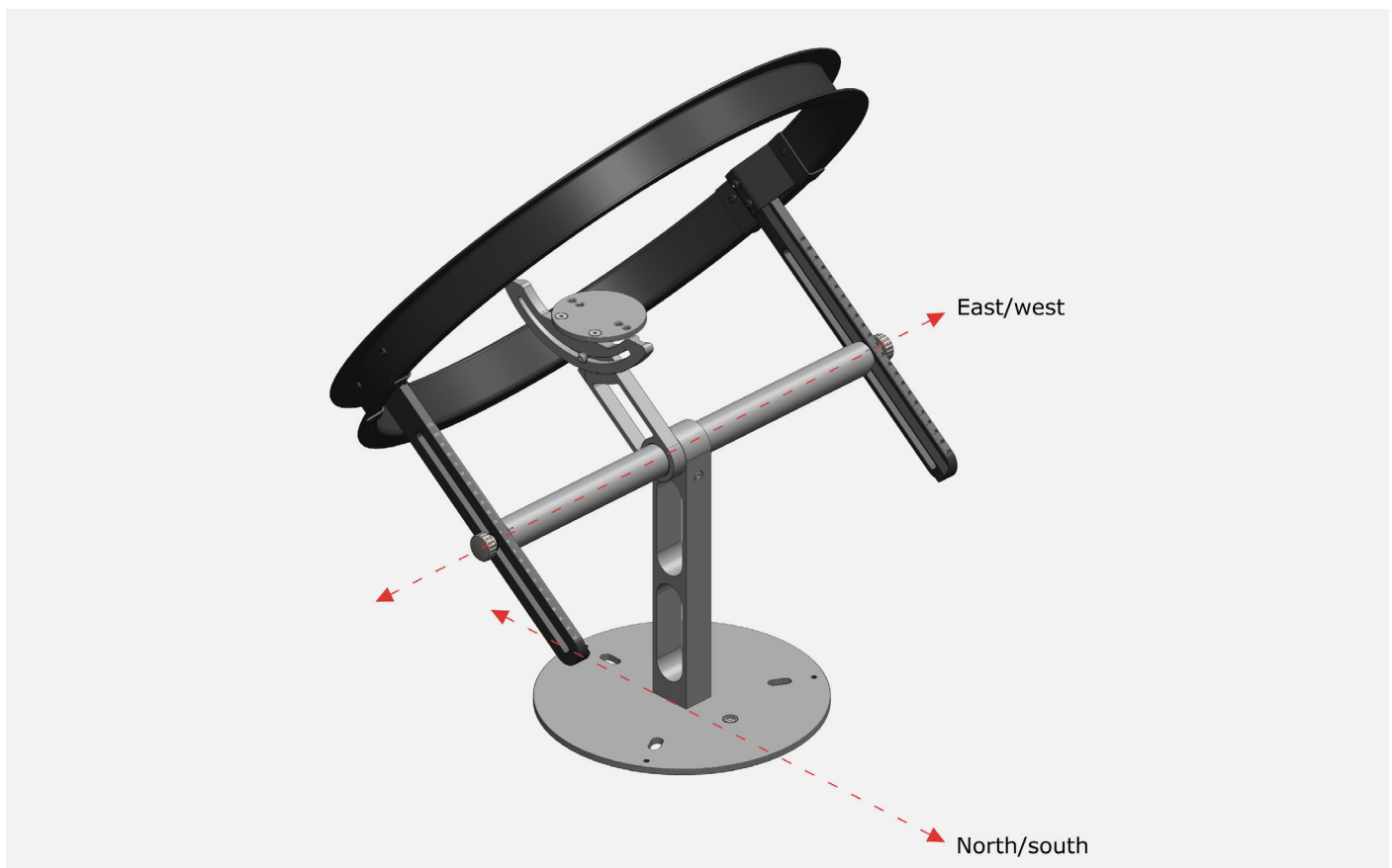
Figure 5.3.1.1 Required orientation of shadow ring.
