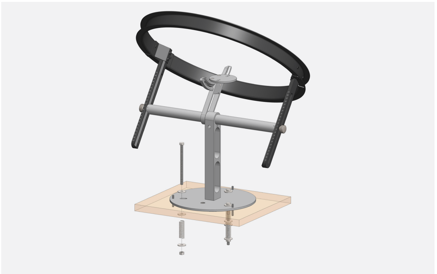
Figure 5.3.2.2 SHR03 mounting fasteners. For easy leveling of the instrument, insert the bolts pointing downwards. Use the washers as shown to keep the springs in place.
