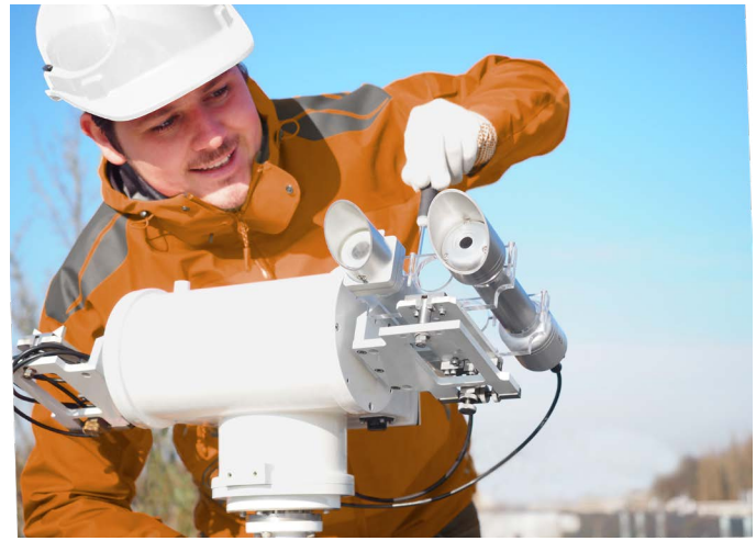
Figure 10 Pyrheliometers with window heating (right) are effective to mitigate snow, frost, and dew deposition on the window, providing the user with more valid data points.
