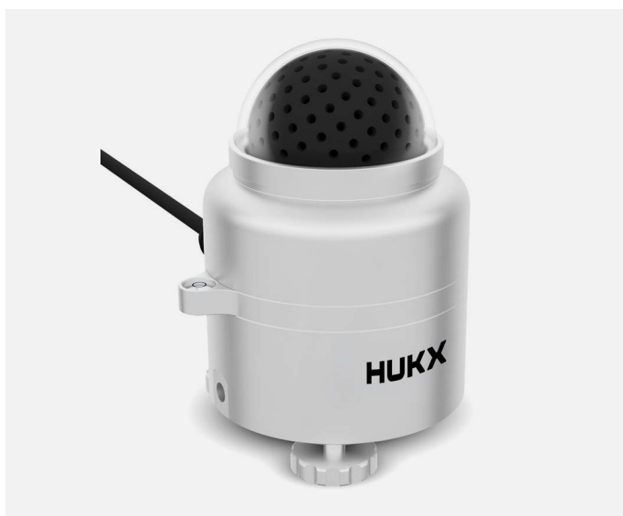
Figure 3 The Hukx SRD100-D1 diffusometer, containing a photodiode array with shadow pattern, measures diffuse irradiance without any moving parts.
