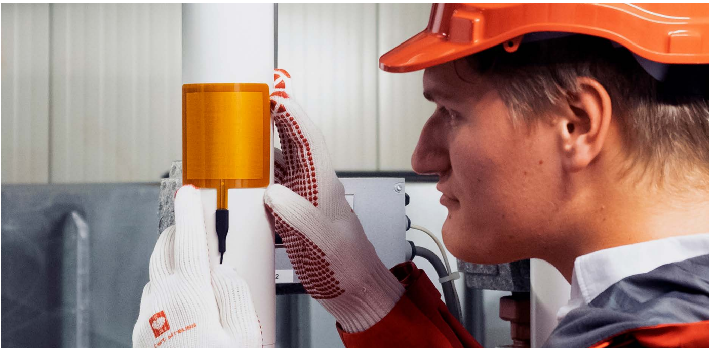
Figure 1 Model FHF05-85X5 heat flux sensor on a pipe to study heat losses.
