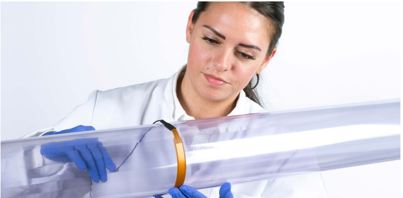
Figure 1 Flexible heat flux sensor model FHF05-15X85 on a tube surface measuring heat flux between the tube and its environment.
