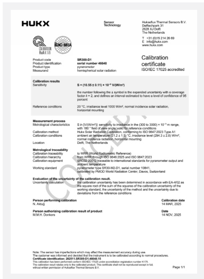
Figure 7 Example of a calibration certificate with each sensor, documenting traceability and uncertainty evaluation.
