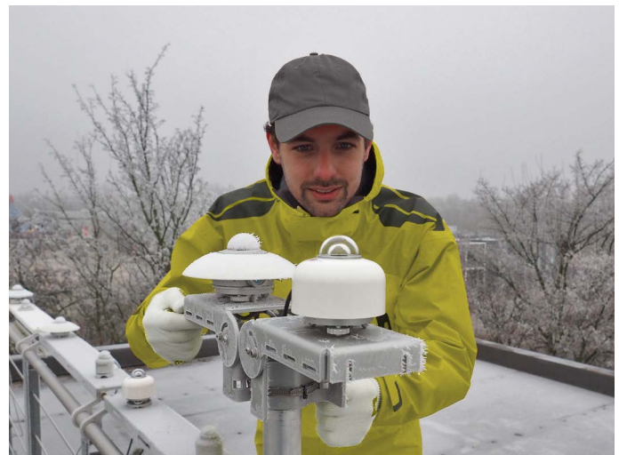
Figure 1 Frost and dew deposition: clear difference between a non-heated pyranometer (left) and SR300 with heating (right).
