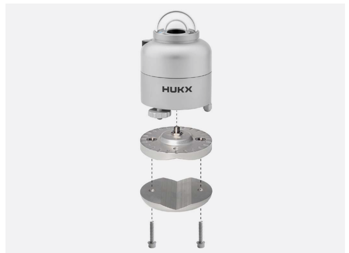
Figure 1 Corrosion protection: Hukx pyranometers, such as SR300-D1, are mounted from below with one bolt that is out of reach for water. No bolts through the housing.
