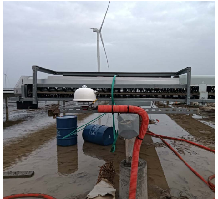
Figure 8 The Hukx SR20 pyranometer with a VU01 ventilation unit at the Khavda PV power plant, next to a waterless cleaning robot.
