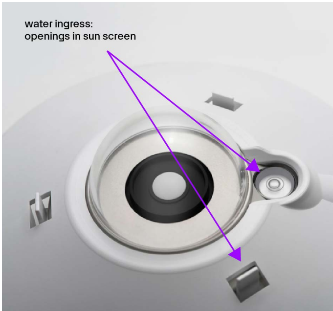
Figure 6 Competing pyranometer with open sun screen. Rainwater and salt spray can pass through openings in the sun screen.
