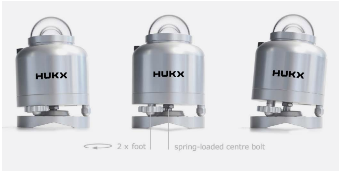
Figure 3 Corrosion protection: the bolt is spring-loaded. No bolts through the housing, that must be loosened when the instrument is levelled.
