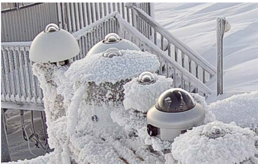
Figure 5 SR30 is battling the elements in Barrow, Alaska, yet the dome remains ice-free. Note that the neighboring, completely ice-free sensors are heated with five times more heating power. Picture taken on 27 JAN 2018 (temperature -30 °C), courtesy of NOAA.
