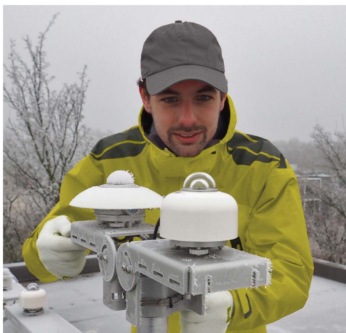
Figure 2 A common issue in freezing conditions: ice accumulation on the dome of a traditional pyranometer (left) reduces data availability. The heated SR30 (right) mitigates this problem.
