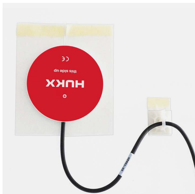
Figure 3 Installation of HFP01 on a wall using 2-sided "removable" carpet laying tape such as TESA 4939 (table 1, NR4) and a strain relief of the cable using a cable tie mount equipped with the same carpet laying tape as adhesive. Note that the optical properties in the visible range do not match those of the surrounding wall. This is acceptable if the heat transfer by visible radiation is negligible, in other words if there is no solar radiation or illumination by strong lamps.
