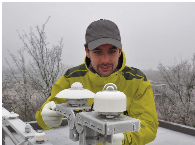
Figure 3 Hukx model SR30 (right) is the first heated pyranometer compliant with the requirements of IEC 61724-1 for Class A monitoring systems. SR30 and the later model SR300 mitigate dew and frost, unlike the non-heated pyranometer on the left. Dew and frost deposition on the pyranometer dome reduce data availability and accuracy.
