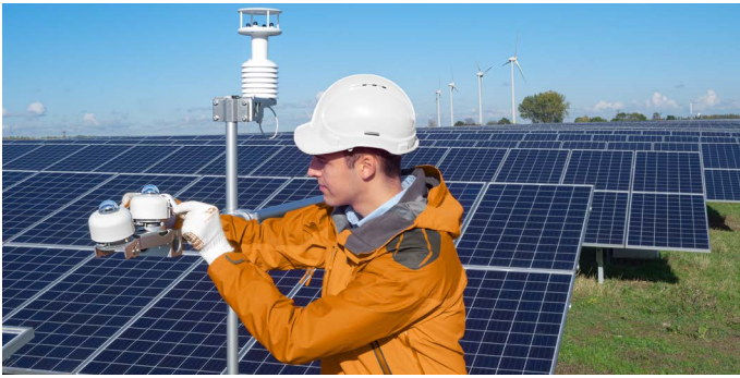
Figure 2 PV system performance monitoring with pyranometers measuring GHI and POA.
