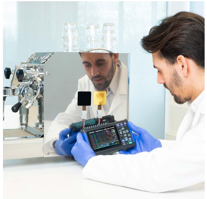
Figure 1 FHF's with BLK and GLD sticker used with Hioki LR8432.
