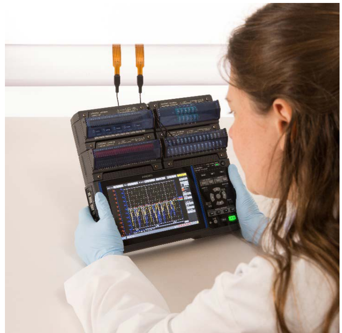
Figure 3 Hioki LR8450-01 can display voltage and temperature data of multiple sensors simultaneously on screen.
