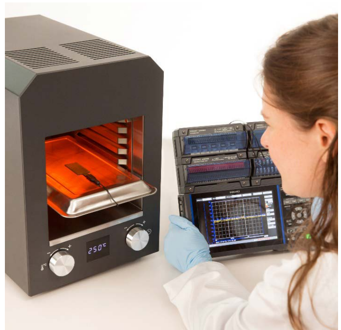
Figure 1 High temperature foil heat flux sensor model FHF06-25X50 used with Hioki LR8450-01.
