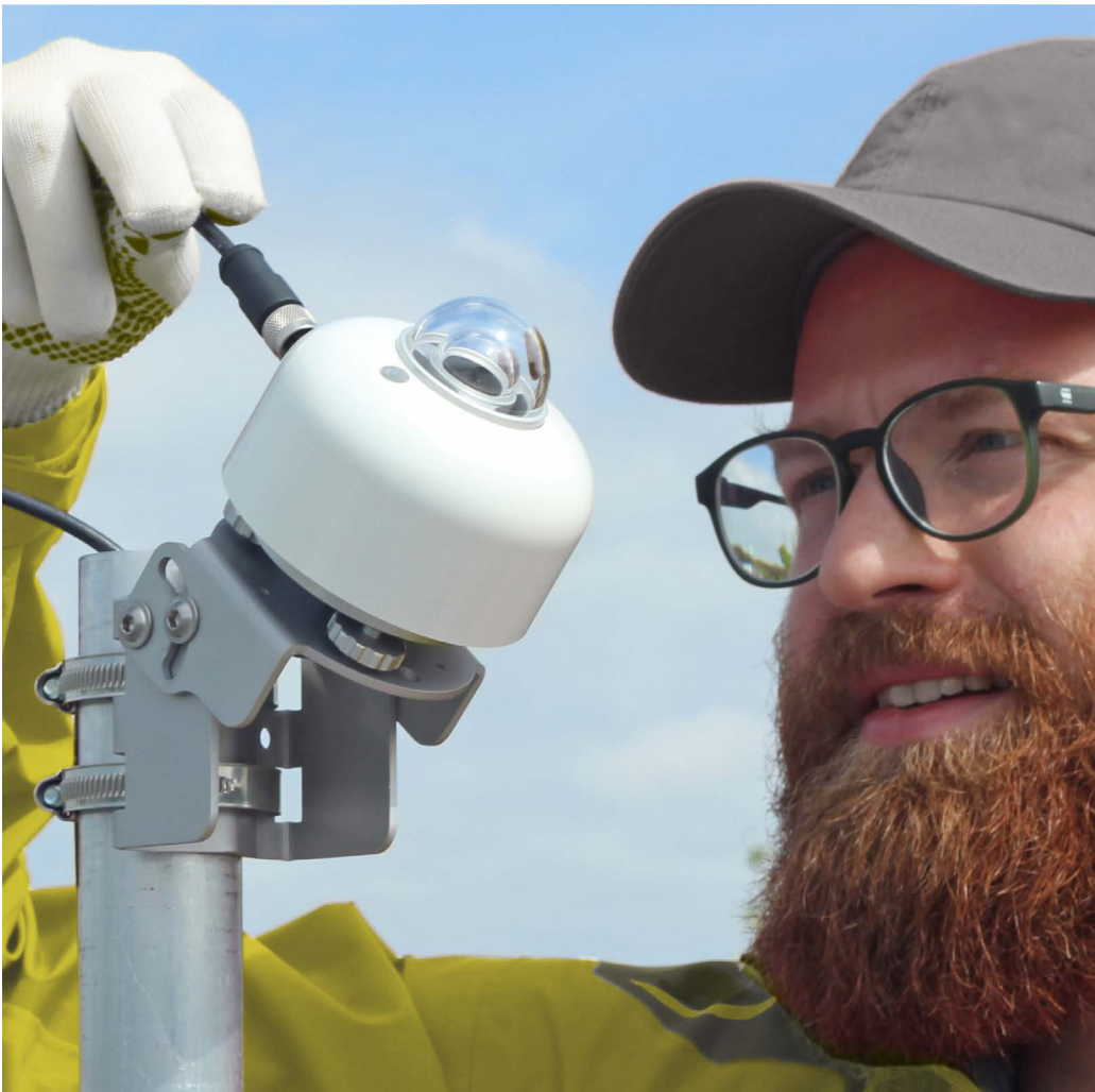
Figure 2 PMF01 pyranometer mounting fixture can be used for easy installation of a pyranometer, in this case SR300-D1, in Plane of Array for PV system performance monitoring and meteorological applications.
