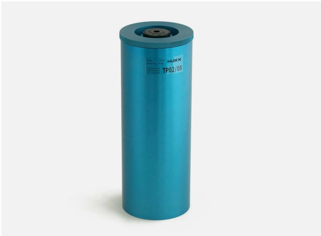
Figure 0.6 A CRC01 calibration reference cylinder containing a polymethylmethacrylate reference material for calibrating TP02 and TP08.
