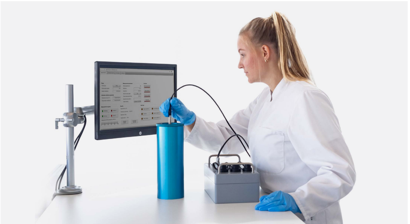
Figure 0.1 Application of the complete TPSYS20 measuring system in a laboratory environment using a CRC01 calibration reference cylinder.
