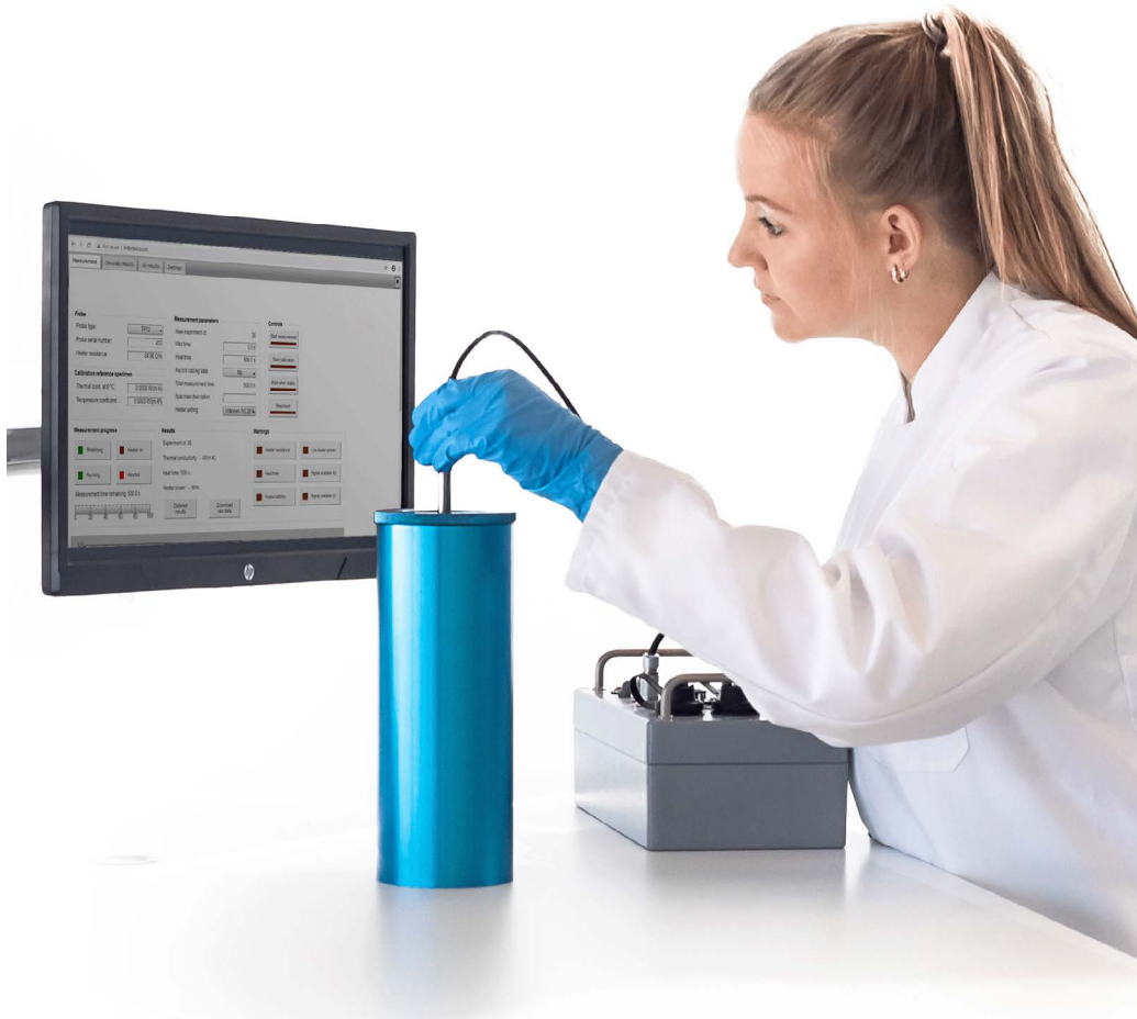
Figure 2 Application of the complete TPSYS20 measuring system in a laboratory environment using a CRC01 calibration reference cylinder.
