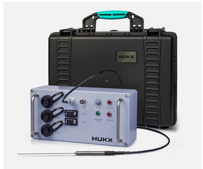
Figure 7 TPSYS20 measuring system includes a TP02/TP08 probe, MCU and carrying case.
