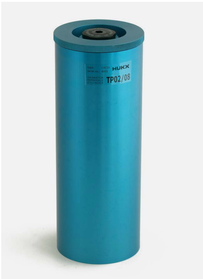
Figure 8 A CRC01 calibration reference cylinder containing a polymethylmethacrylate reference material for calibrating TP02 and TP08.
