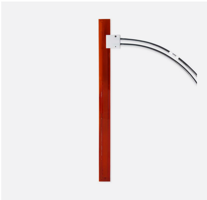
Figure 5 STP01 soil temperature profile sensor which is often combined with TP01 for soil energy budget calculation.
