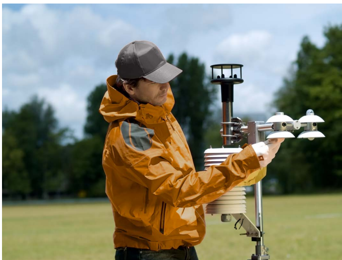
Figure 2 TP01 is typically used in high-accuracy surface flux measurement stations.
