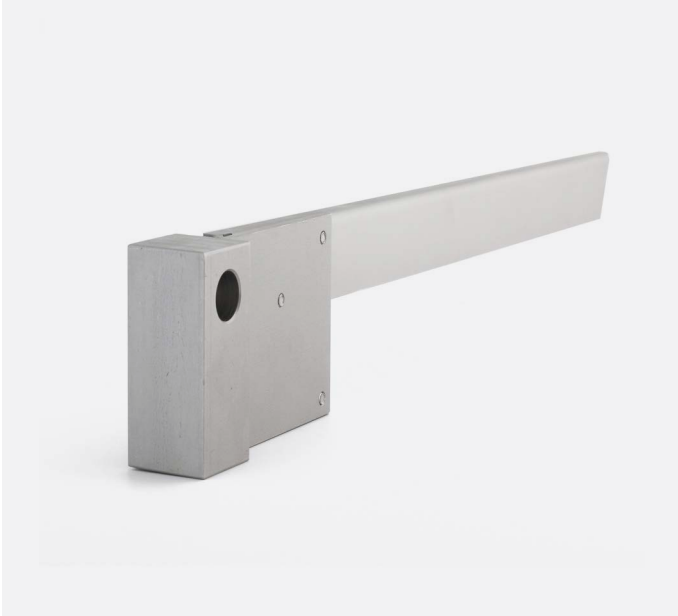
Figure 4 IT01 insertion tool is hammered down into the soil. After retracting it leaves a slit in which STP01 may be inserted.
