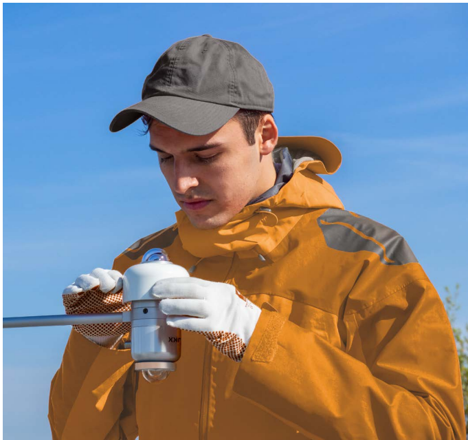
Figure 4 Using the SRA300-D1 albedometer is easy; the instrument is composed of one AMF03 and two SR300-D1 pyranometers.
