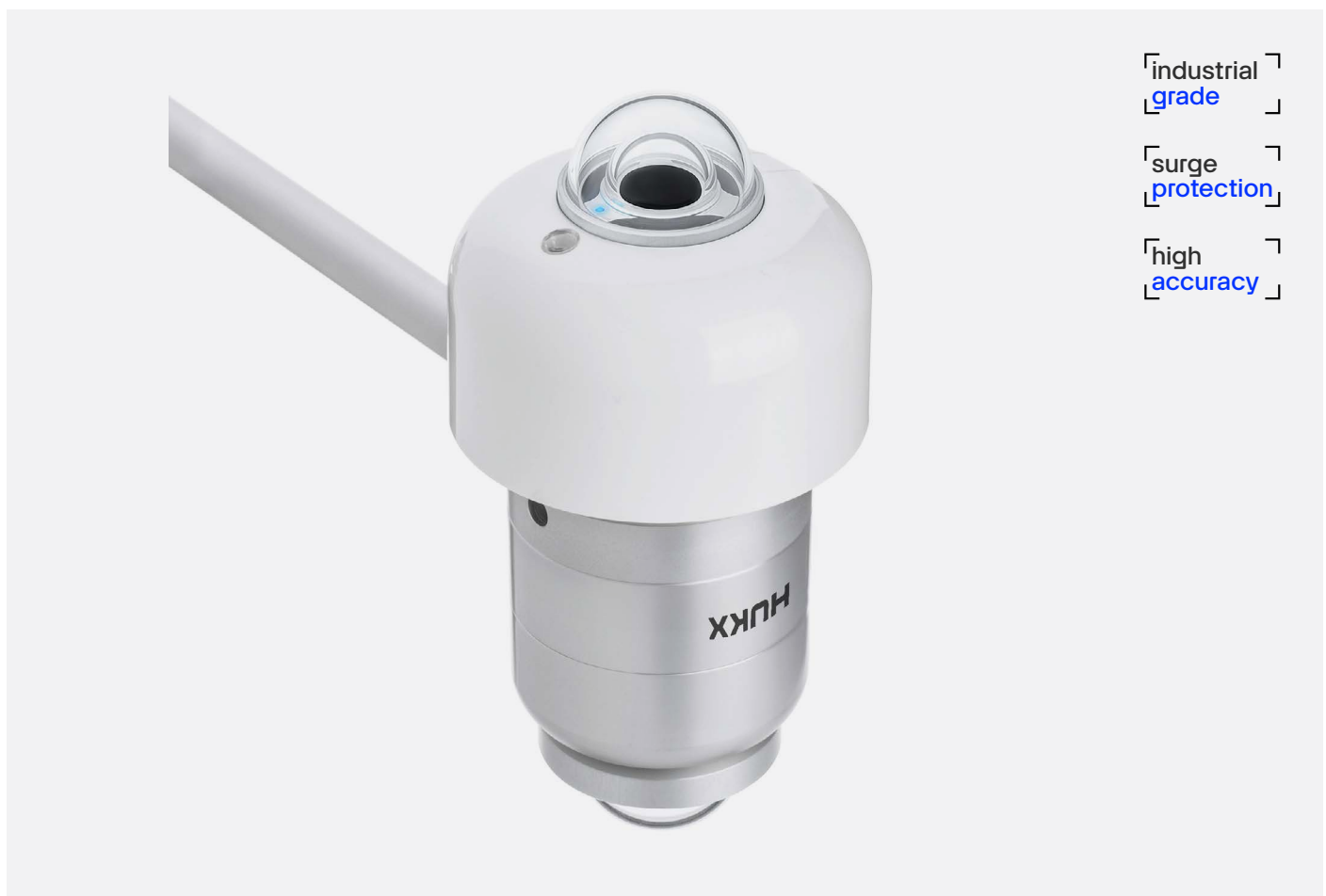
Figure 1 Industrial albedometer model SRA300-D1.
