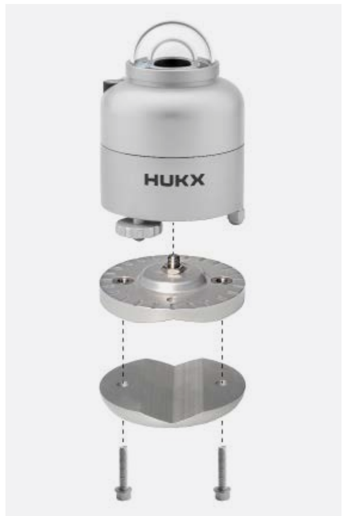
Figure 5 Optional LM01 spring-loaded leveling mount (one part) and TLM01 tube leveling mount (2 parts) for SR300-D1, SR200-D1, and SR100-D1. Spring-loaded leveling is a major time-saver during installation.
