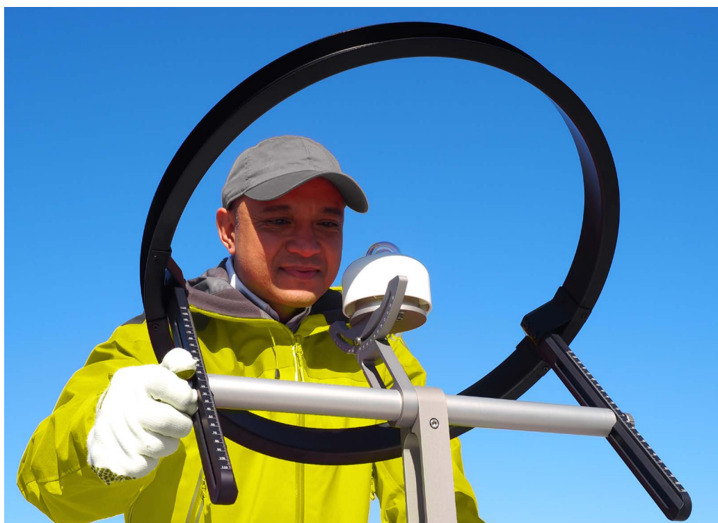
Figure 0.2 Installation of the SHR02 shadow ring with a Hukx pyranometer is easy.
