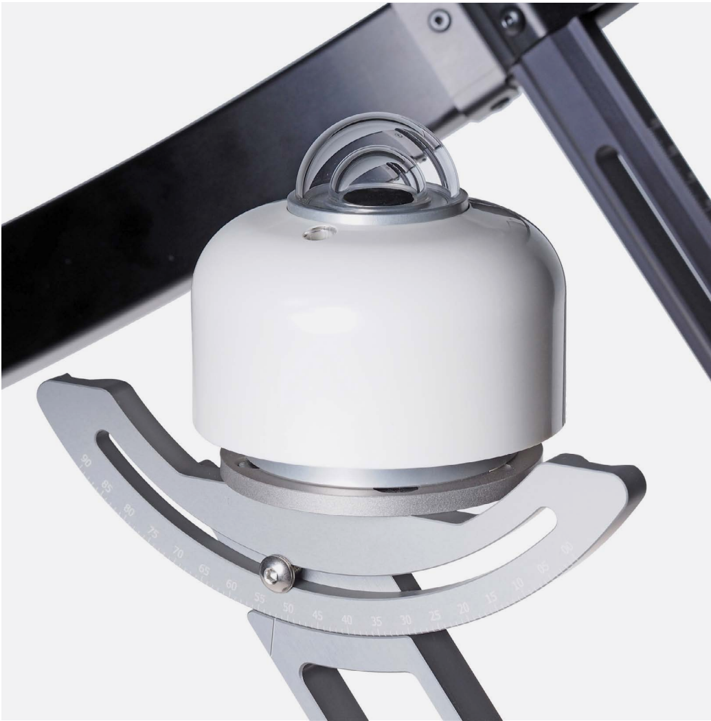
Figure 0.3 Pyranometer example: SR15, combined with SHR02 forming a diffusometer.
