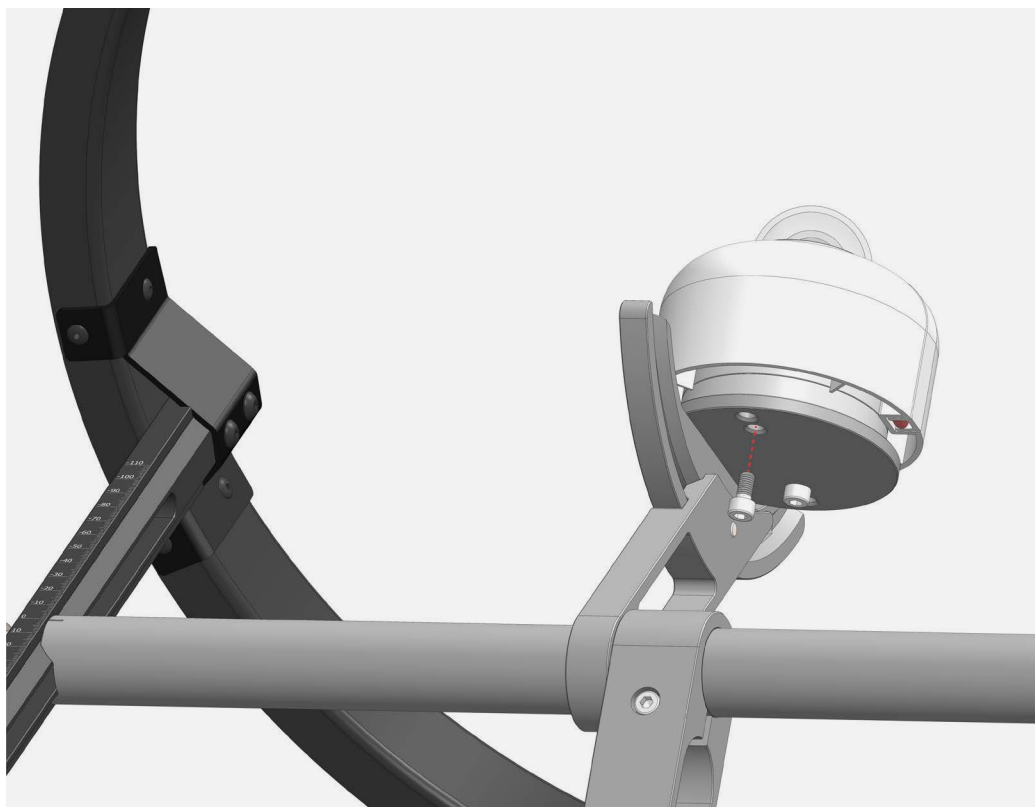
Figure 5.4.3.1.1 Mounting an SR15 pyranometer on SHR02.
