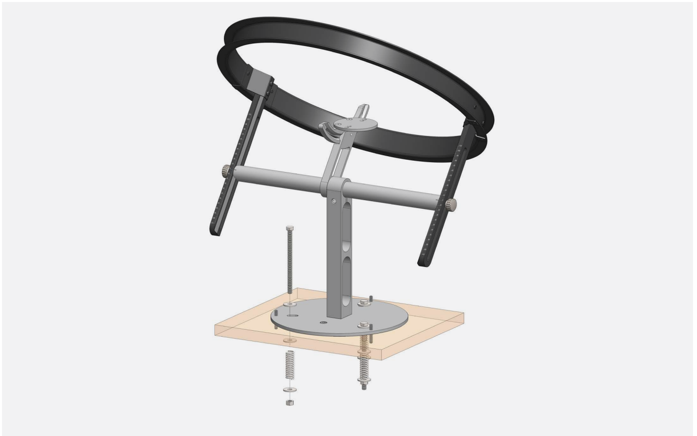
Figure 5.3.2.2 SHR02 mounting fasteners. For easy leveling of the instrument, insert the bolts pointing downwards. Use the washers as shown to keep the springs in place.
