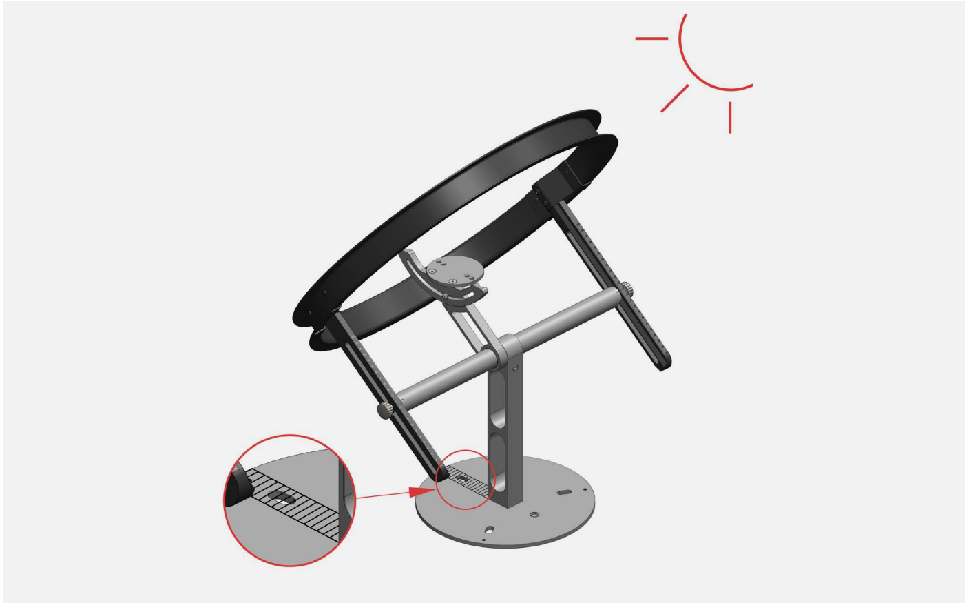
Figure 5.4.1.3.1 Aligning the shadow parallel to the vertical support.
