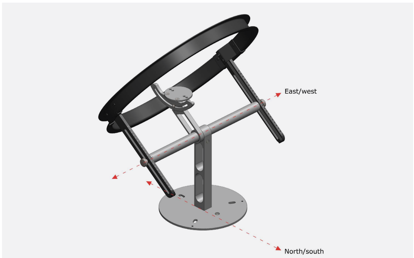
Figure 5.3.11 Required orientation of shadow ring.
