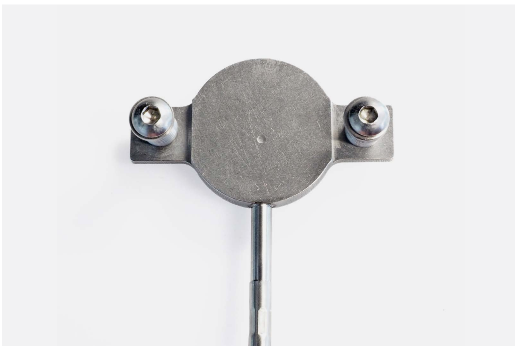
Figure 0.2 IHF01 industrial heat flux sensor ready for mounting on a well-prepared surface using tack-welded threads and spring-loaded bolts.
