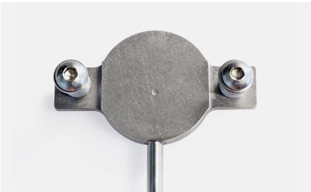
Figure 5.11 Installation of IHF01 with spring-loaded bolts (not included with IHF01) using tack-welds on a well-prepared flat surface.
