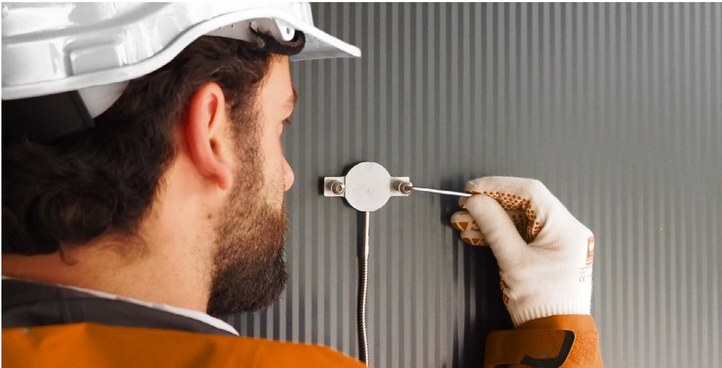
Figure 4.11 Example of an IHF01 industrial heat flux sensor mounted on a wall using spring-loaded bolts and tack-welded threads. The sensor is mounted on a well-prepared flat surface.
