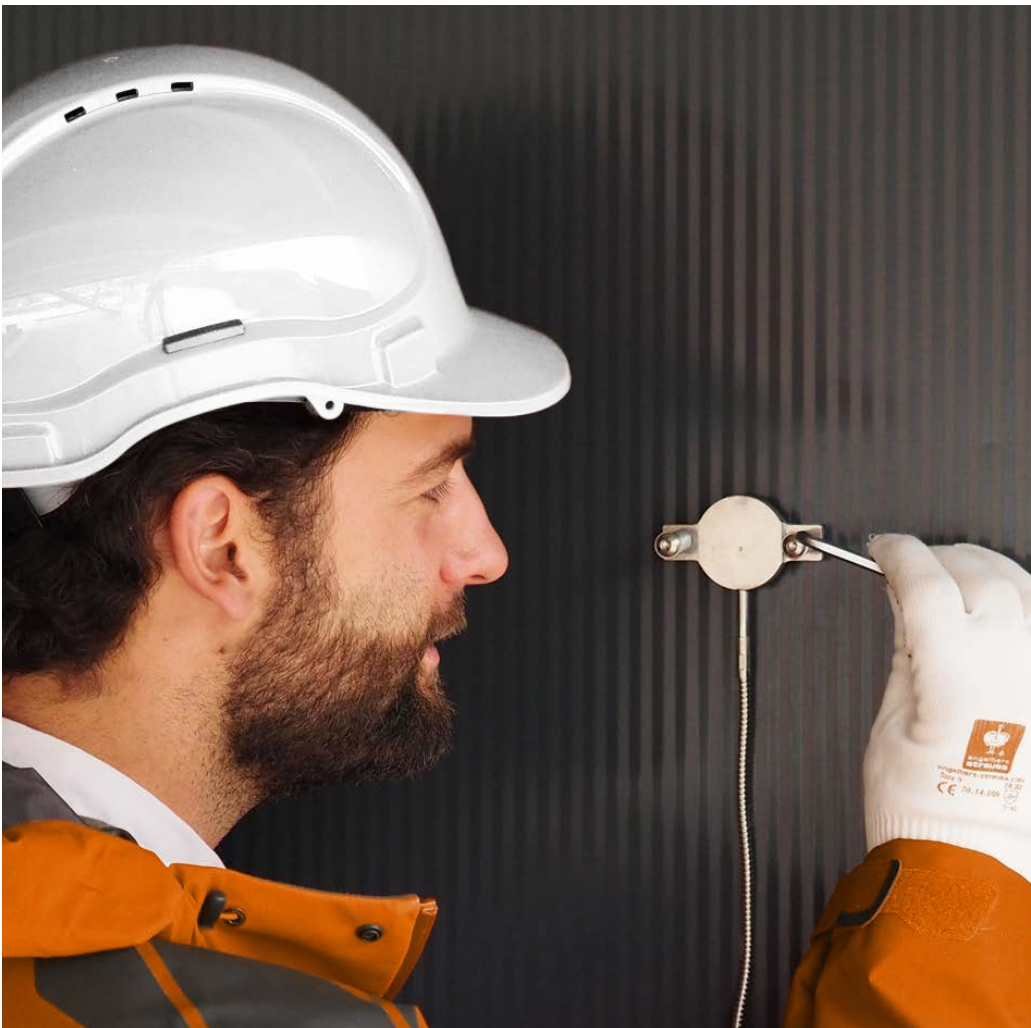
Figure 2 Example of an IHF01 industrial heat flux sensor mounted on a wall using tack-welded threads and spring-loaded bolts.
