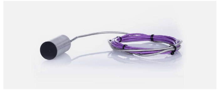
Figure 4 HFS01, pictured without flange and with cabling.
