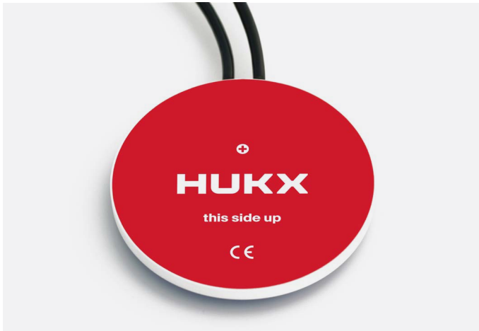
Figure 0.1 HFP01SC self-calibrating heat flux sensor. The opposite side has a blue cover.
