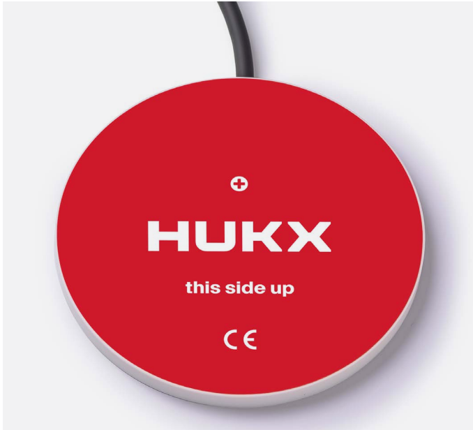
Figure 0.1 HFP01 heat flux plate/sensor. The opposite side has a blue-colored cover.
