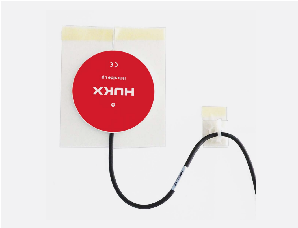
Figure 5.11 Installation of HFP01 on a wall using sided “removable” carpet laying tape such as TESA 4939, and a strain relief of the cable using a cable tie mount equipped with the same carpet laying tape as adhesive.
