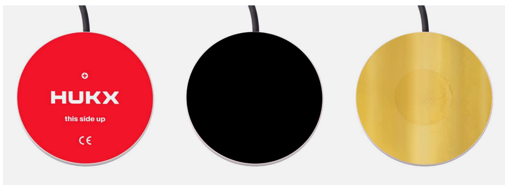
Figure 0.3 HFP01 heat flux plate with BLK-80 and GLD-80 stickers to measure radiative and convective heat fluxes separately.
