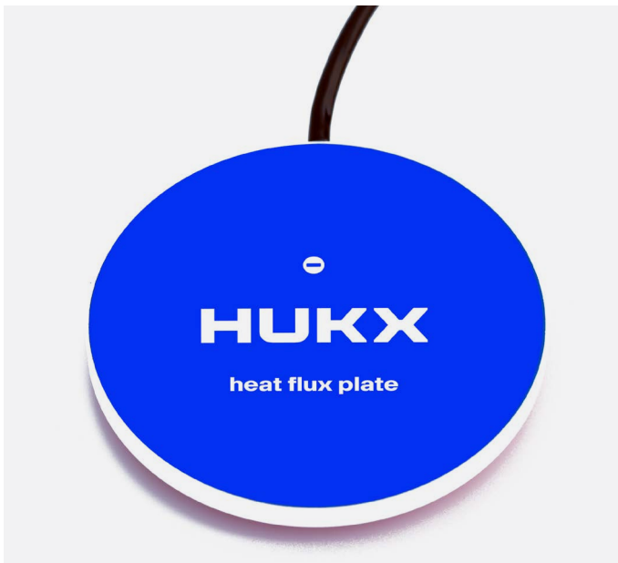
Figure 0.2 HFP01. The opposite side has a red-colored cover. Standard cable length is 5 m.
