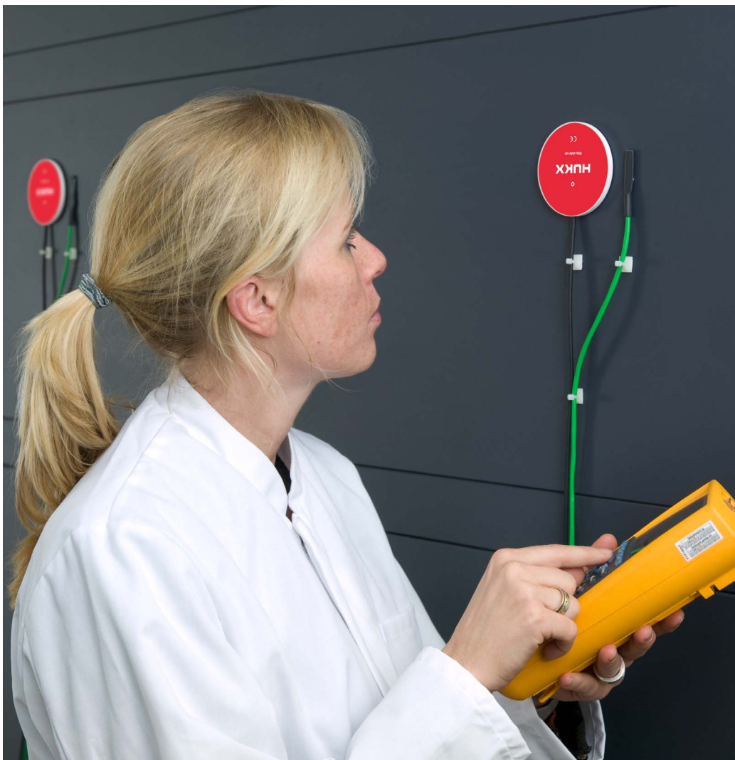
Figure 4.1.1 HFP01 heat flux sensors in use on a wall.
