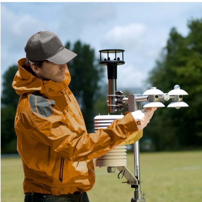
Figure 4.21 Typical meteorological surface energy balance measurement system with HFP01 installed under the soil.
