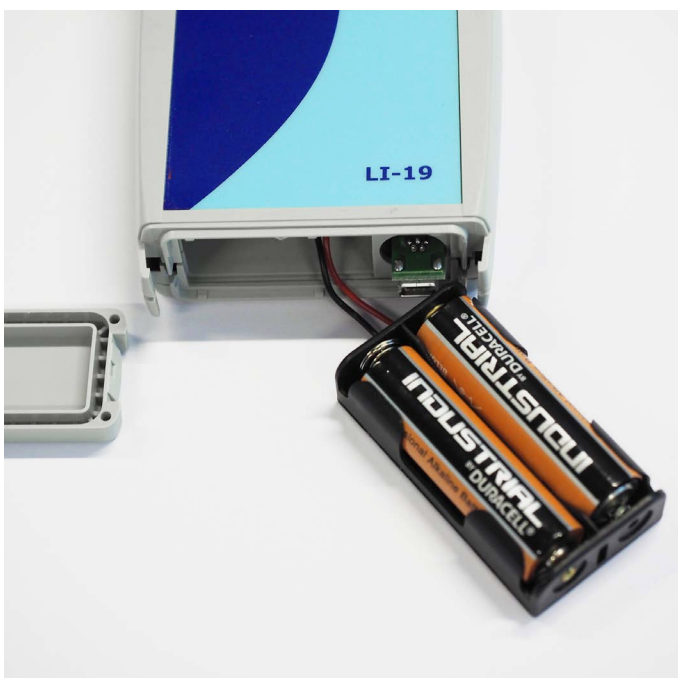
Figure 5.3.1 Battery replacement of LI19.
