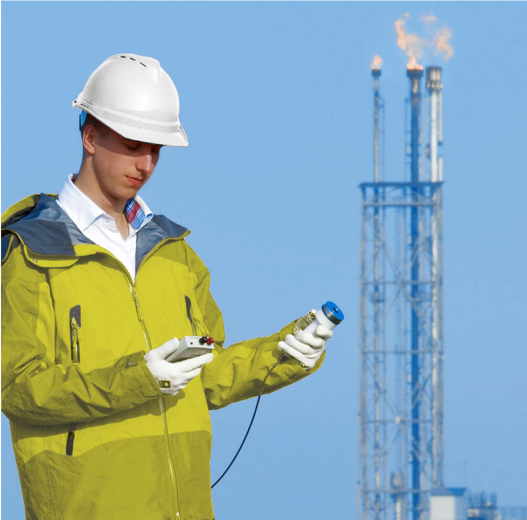
Figure 0.3 HF03-LI19 portable heat flux sensor with read-out unit in use for studying flares.
