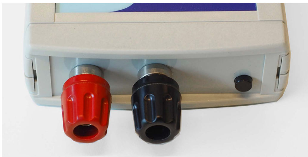
Figure 4.1.1 Connectors and on/off switch on LI19. Connectors are 2 x female chassis plugs for 4 mm banana plug, with screwed signal wire clamps
