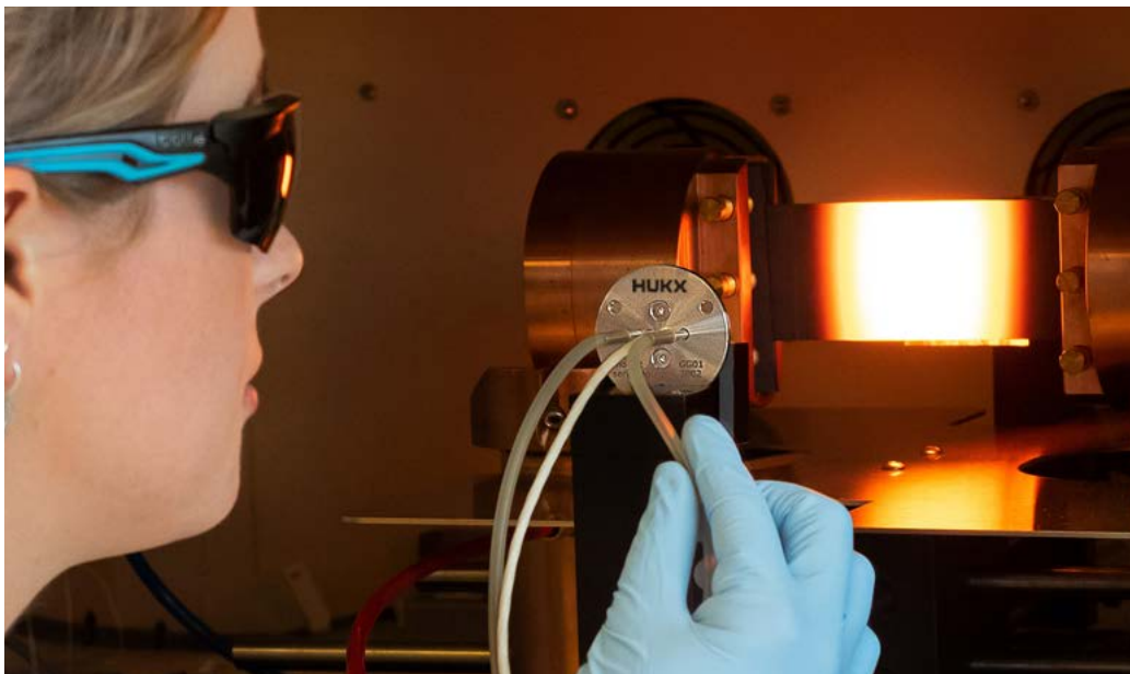
Figure 2 GG01 sensor in a high heat flux test cabinet. Each sensor is tested at its rated measurement range.
