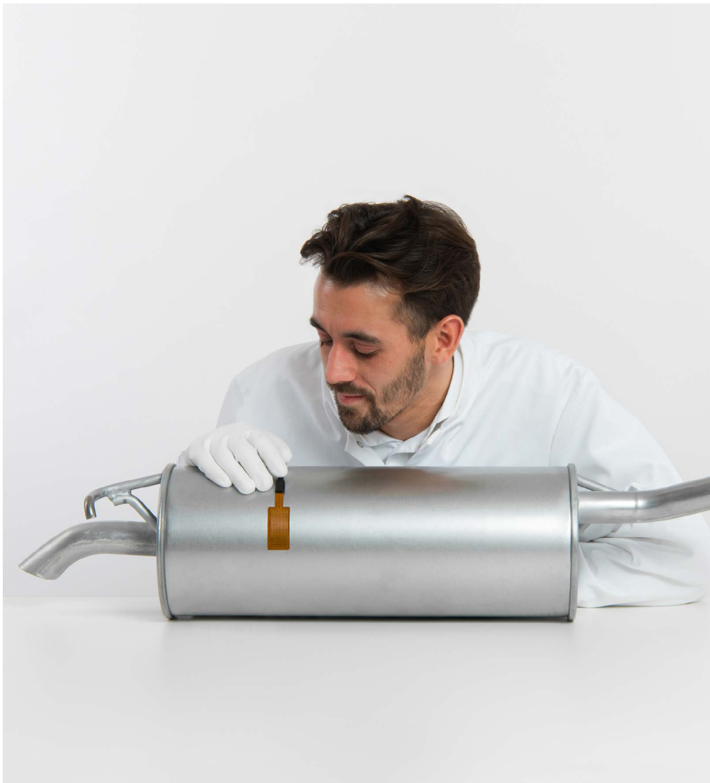
Figure 4.11 Example of model FHF06 high temperature foil heat flux sensor being installed for measurement on a car exhaust. FHF06 is flexible and can be easily mounted on a curved surface like a pipe or tube.
