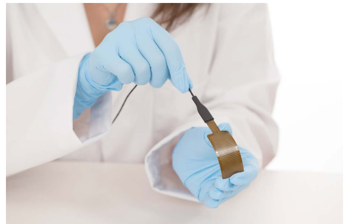
Figure 3 The thin and flexible FHF06 can be easily mounted on a curved surface, like a pipe or tube.
