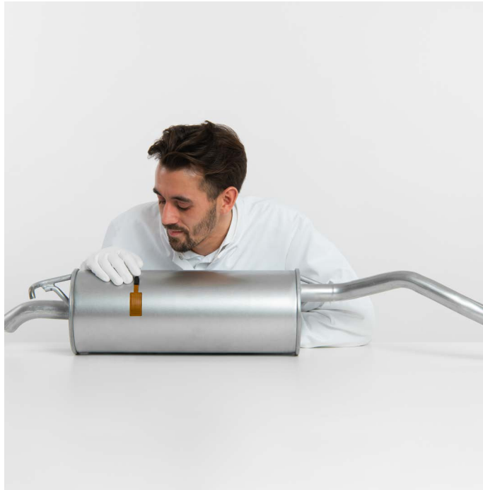
Figure 2 FHF06 high-temperature foil heat flux sensor installed for measurement on a car exhaust pipe. The sensor may be mounted on a curved surface.
