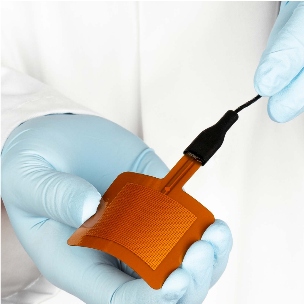
Figure 2.1.2 Heat flux from the backside to the frontside generates a positive voltage output signal. The dot on the foil indicates the frontside. The backside of the FHF05SC has a heater.
