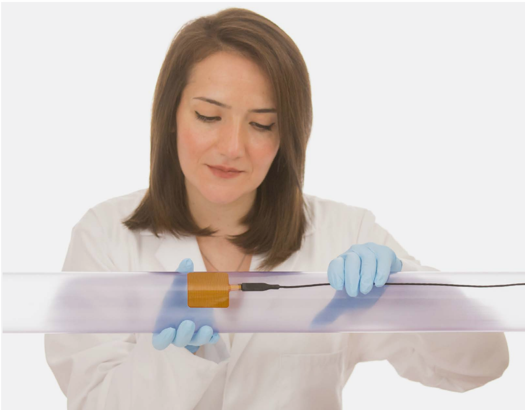
Figure 5.31 Bending of model FHF05SC-50X50 foil heat flux sensor, in this image on a pipe.
