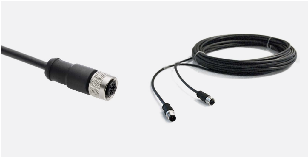
Figure 0.3 On the left, the DR30-D1 cable with M12-A female connector on sensor end, pigtails of 0.15 m and conductors with ferrules. Its length is 5 meters standard and available in 10 and 20 meters too. On the right, the optional Hukx extension cable with connector pairs, with male and female M12-A connectors, available in 20 meters.
