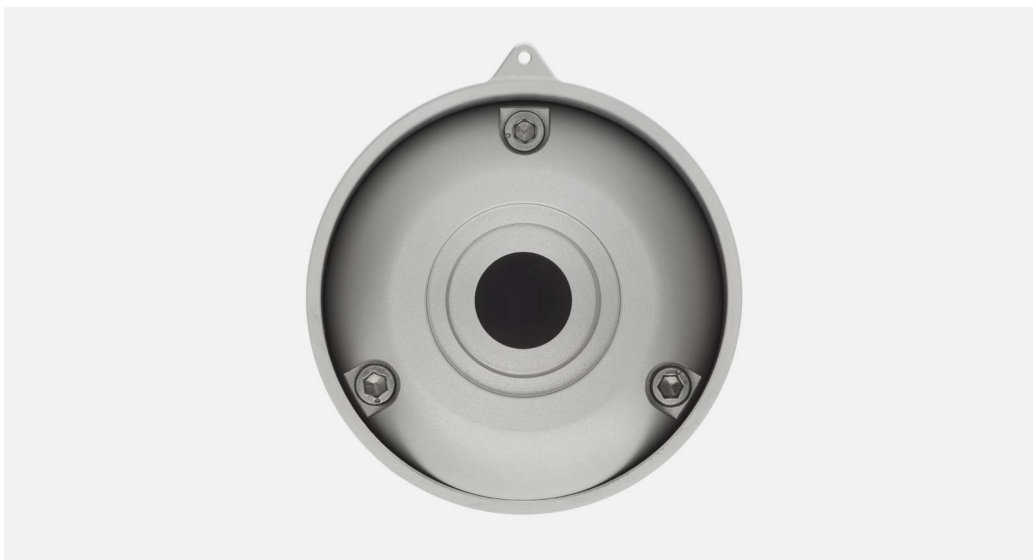
Figure 1.3.1 DR30 first class pyrheliometer front-view; window assembly with heater.
